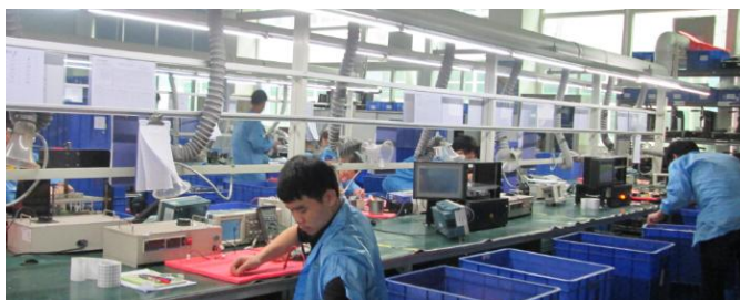
Electrical parts testing with automation fixtures. Every units of drive has tested with load before factory leaving
