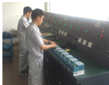
Electrical parts testing with automation fixtures. Every units of drive has tested with load before factory leaving
